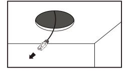
2. Then plug the RJ45 cable into the speaker. Once connected, make sure to close the carrying case with the cover provided.
