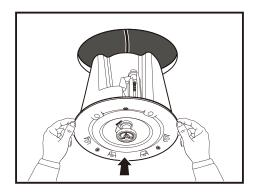
**Note:** Do not press the small drive unit in the front center of the speaker, this will damage the speaker.
