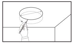
**Warning:** The thickness of the ceiling should not exceed 30mm, and do not cut into the surface when drawing the outline, so as not to damage the wires or pipes on the back and cause safety hazards. If you are not sure about your ability to install this speaker yourself, please contact a professional installer for on-site installation.
