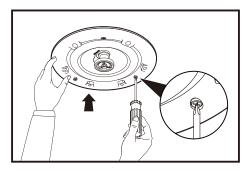
Note: If using a power drill, choose the lowest torque setting.
